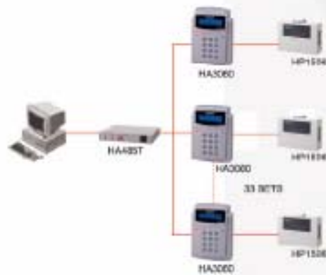
Network configuration upto 32 sets with HA305 connected
